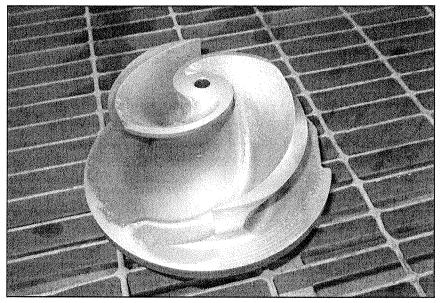
• Impeller is in good condition and will be reused.
